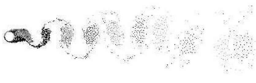
Fig. 5. Wake visualization, V_r = 2.00 .
